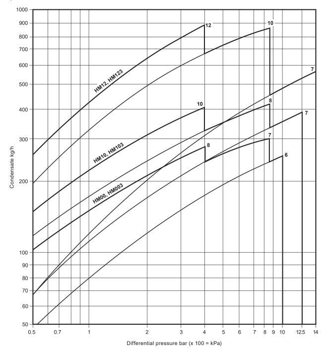
Note: Traps should be selected for the most appropriate working pressure differential and not on the basis of load.
